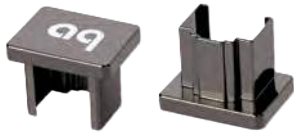
RJ45 Noise-Stopper Caps AQ Noise-Stopper Caps fit over unused RJ45 inputs or outputs, preventing RFI and EMI noise from entering the active circuit. Noise-Stopper Caps also protect against dust and corrosion.
